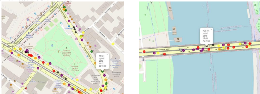
Figure 1. Example of finding timestamped geolocated hotspots and coldspots a) weekday night in city center (Vukov spomenik), PM 10 ~14µg/m 3 , b) workday early afternoon in city center (Brankov most), PM 10 ~400µg/m 3
