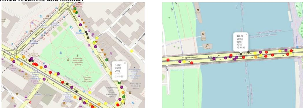
Figure 1. Example of finding timestamped geolocated hotspots and coldspots a) weekday night in city center (Vukov spomenik), PM<sub>10</sub>~14µg/m<sup>3</sup>, b) workday early afternoon in city center (Brankov most), PM<sub>10</sub>~400µg/m<sup>3</sup>
