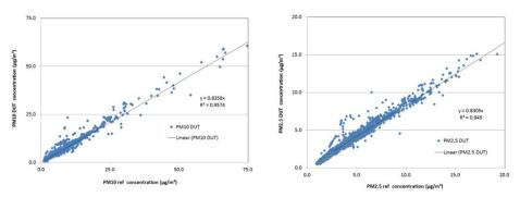
Figure 1. Comparison of results for the PM concentrations measured in the laboratory
