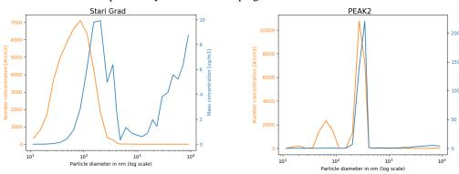
Figure 1. Examples of emission profiles for PM number concentration peaks a) recorded in vehicle campaign b) recorded in small boat campaign
