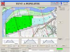
Fig. 8. Ash disposal site TNTA, dry 25% of active area white painted, blue pond
