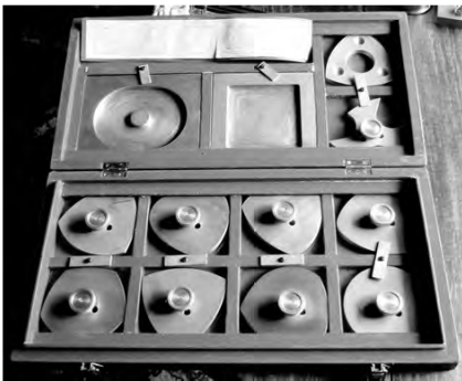
Figure 10.5. A collection of shapes of constant width by G. J. H. Cordle as a final year undergraduate project in 1995.
